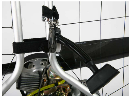
Example of pull start handle mounting on a Bailey Aviation paramotor
